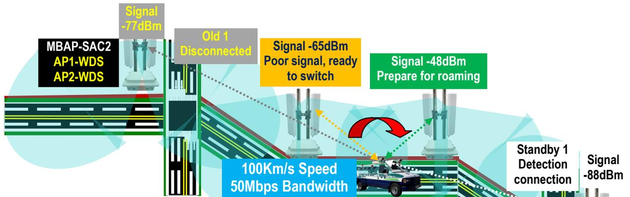
■ Ultra-fast roaming switching mobile wireless transmission function
