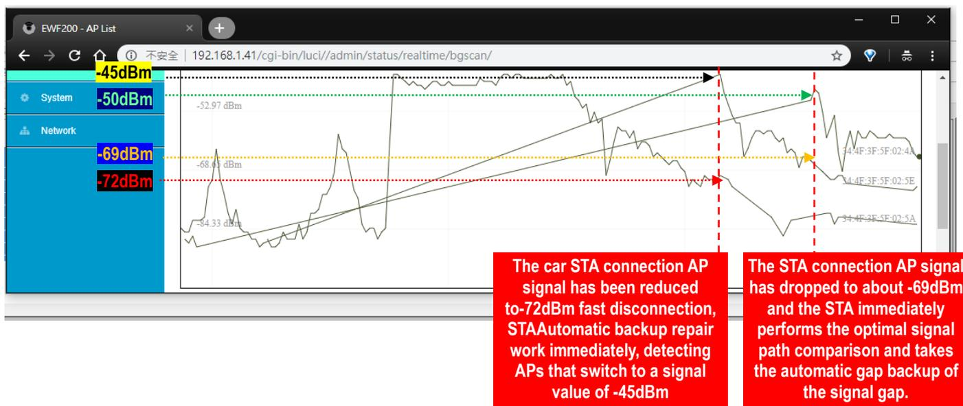
■ After the STA operation mode starts the high-speed mobile function, the mobile terminal STA supports "Super-fast roaming switching mobile wireless transmission function":( Super-Fast Roaming Mobility Features)
