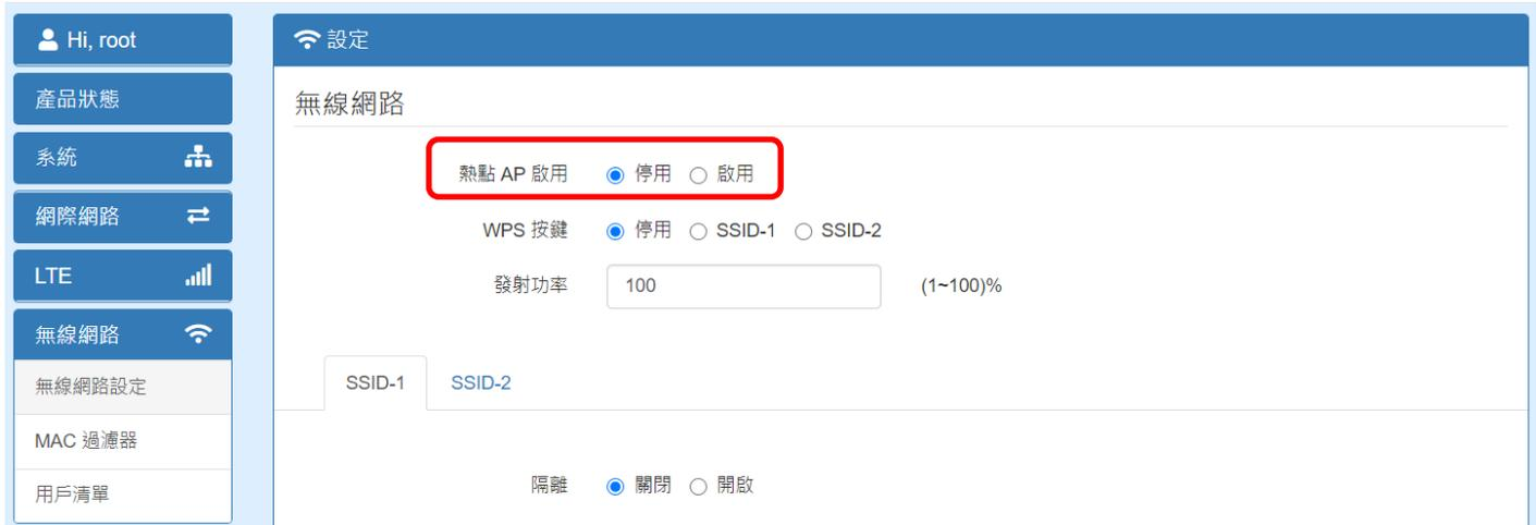
The screenshot shows the '無線網路' (Wireless Network) settings page. The '熱點 AP 啟用' (Hotspot AP Enabled) option is selected as '停用' (Disabled). Other settings include WPS 按鍵 (WPS Button) set to '停用', 發射功率 (Transmit Power) set to 100 (1~100)%, and 隔離 (Isolation) set to '關閉' (Off).
