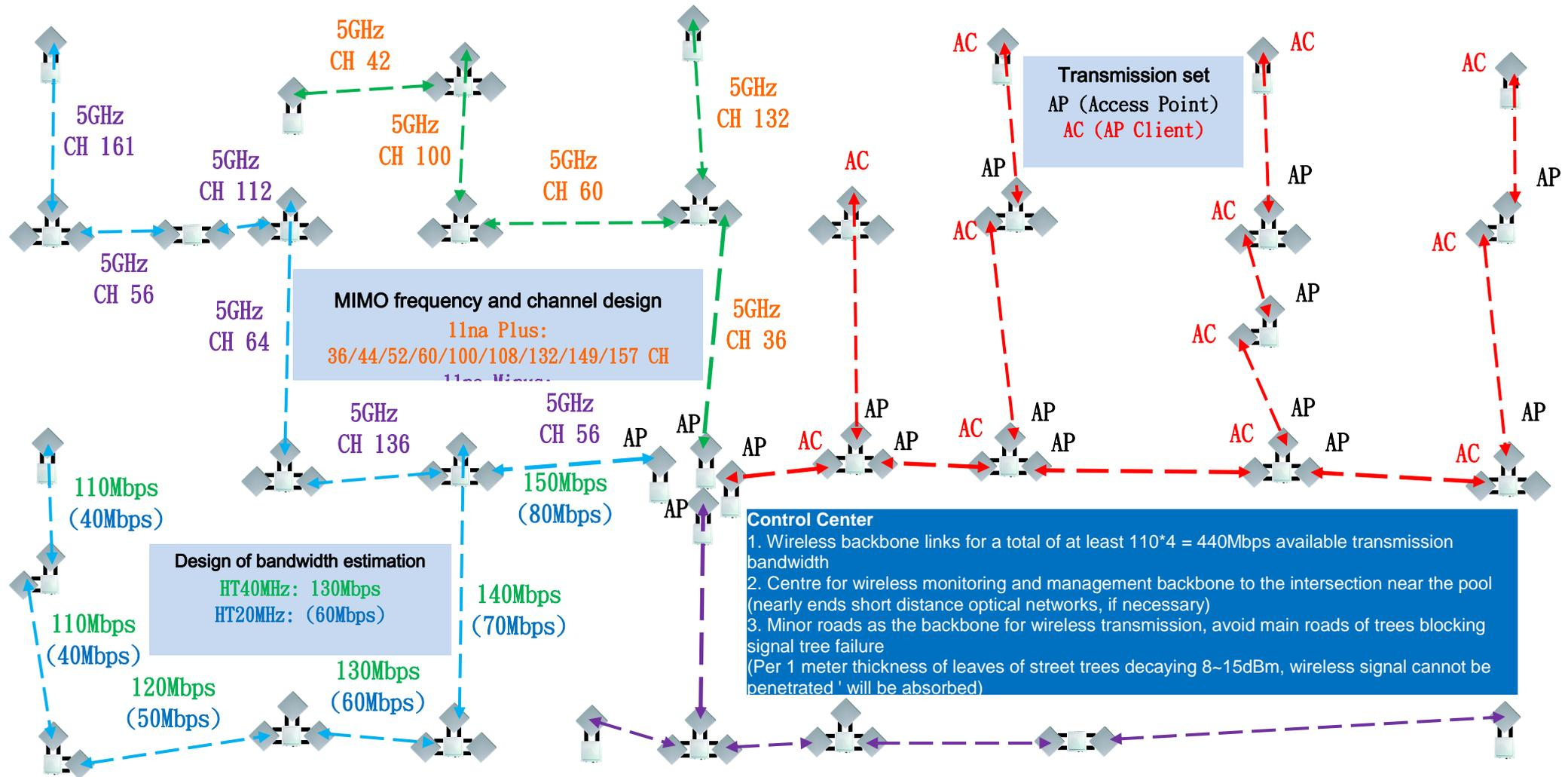
Wireless bandwidth prediction commentary: 1. the multiple hops relay platform technology, 1th hop 140~160Mbps, 2nd hops 130~150Mbps, 3rd hops 120~140Mbps, 4th hops 110~130Mbps, 5th hops after to maintain 110~120Mbps bandwidth, lower bandwidth will not increase the number of platform and response time not less than 10ms.
