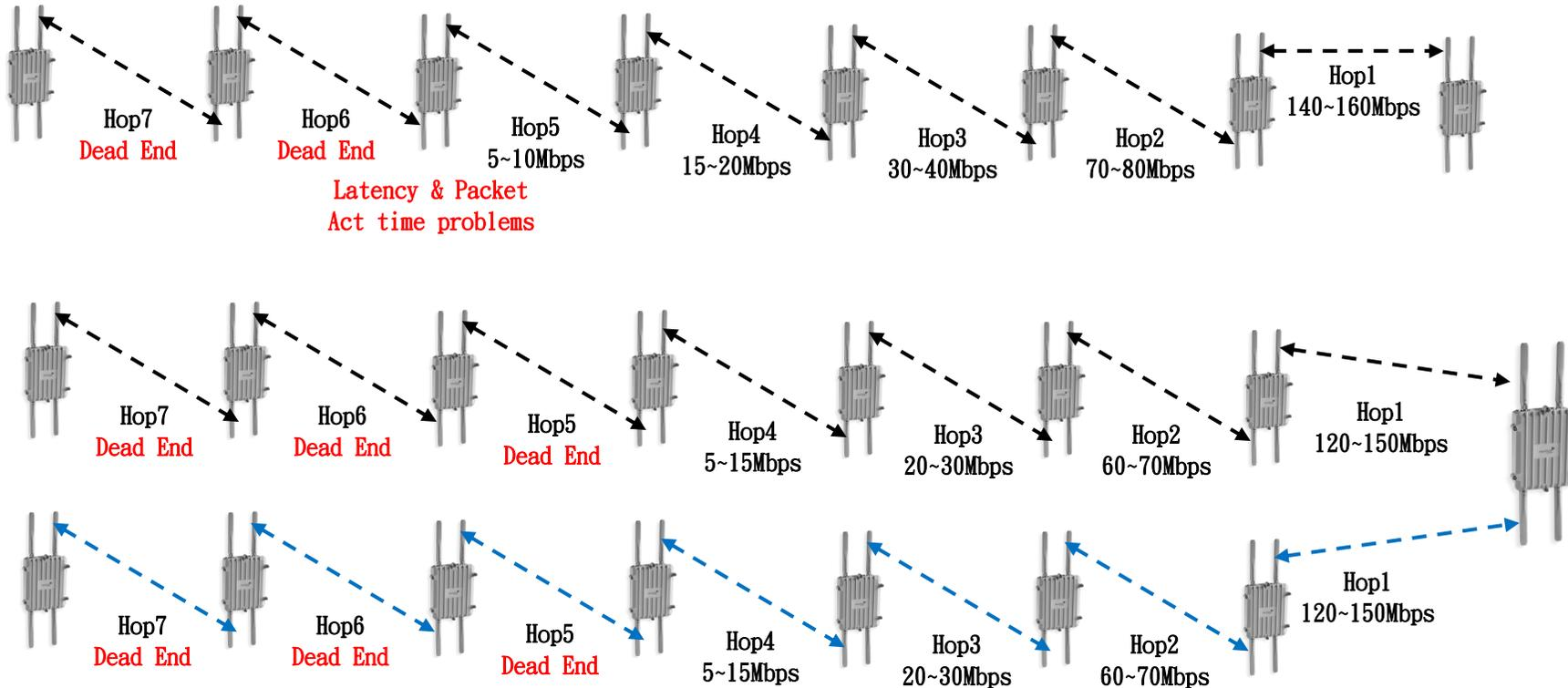
1. Dual RF Module Bridge each hop will reduce 1/3~1/2 throughput. After 5 hops, it may cause backhaul dead end.
