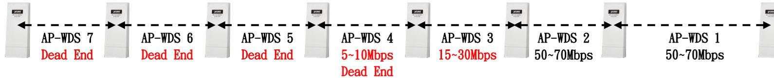
1. AP-WDS is working as AP & AP Client, it is specially extended surf internet backhaul, but the throughput will cut down 1/2 in the backhaul because the devices need to transmit AP-throughput and AP Client-throughput, the total throughput will be shared.
