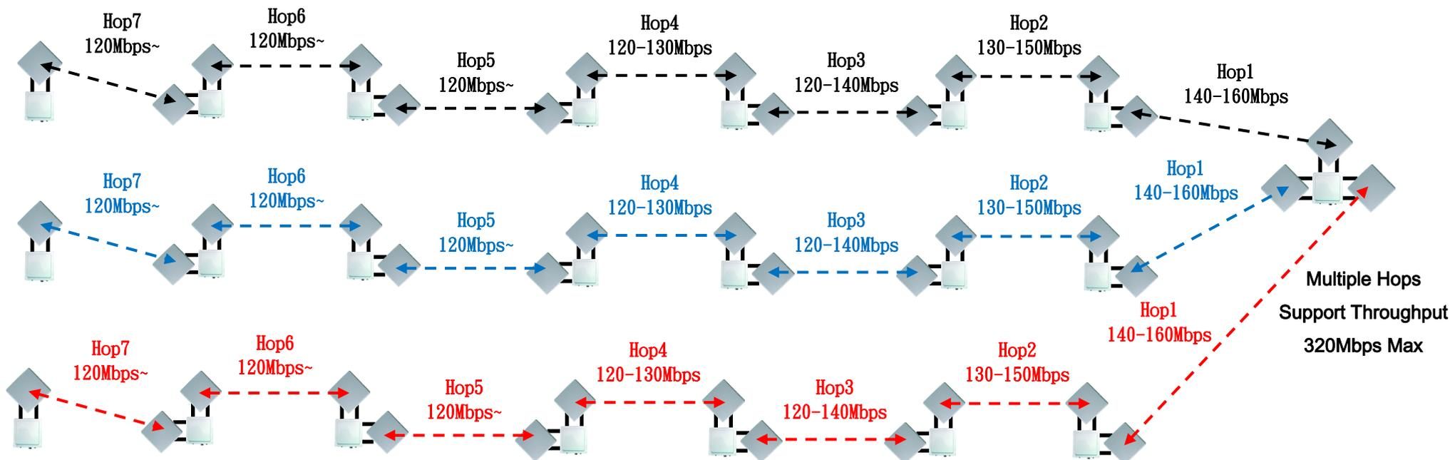
1. Design 2.4GHz & 5.8GHz dual band & 2\*2 MIMO Multi three RF modules backhaul system solution.
