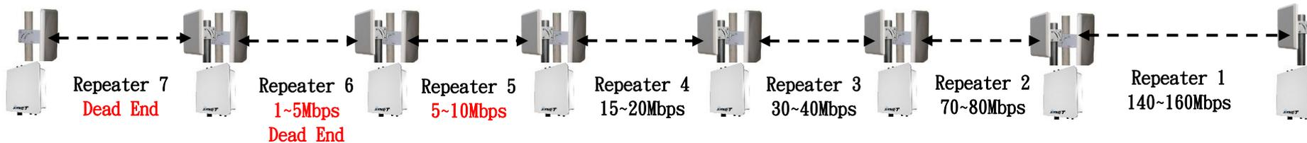
1. Repeater is working as forward transmit, it is specially extended backhaul, but the throughput will reduce 1/2 throughput at each repeater in the backhaul. Even you set up dual radio for wireless repeater system, the throughput will reduce more and faster.
